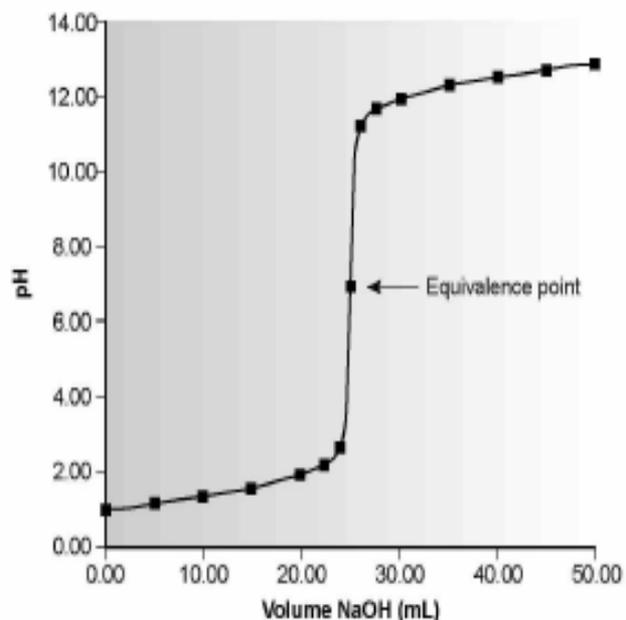
Acid-base titration curve for 25.0 mL of 0.100 M HCl with 0.100 M NaOH.
