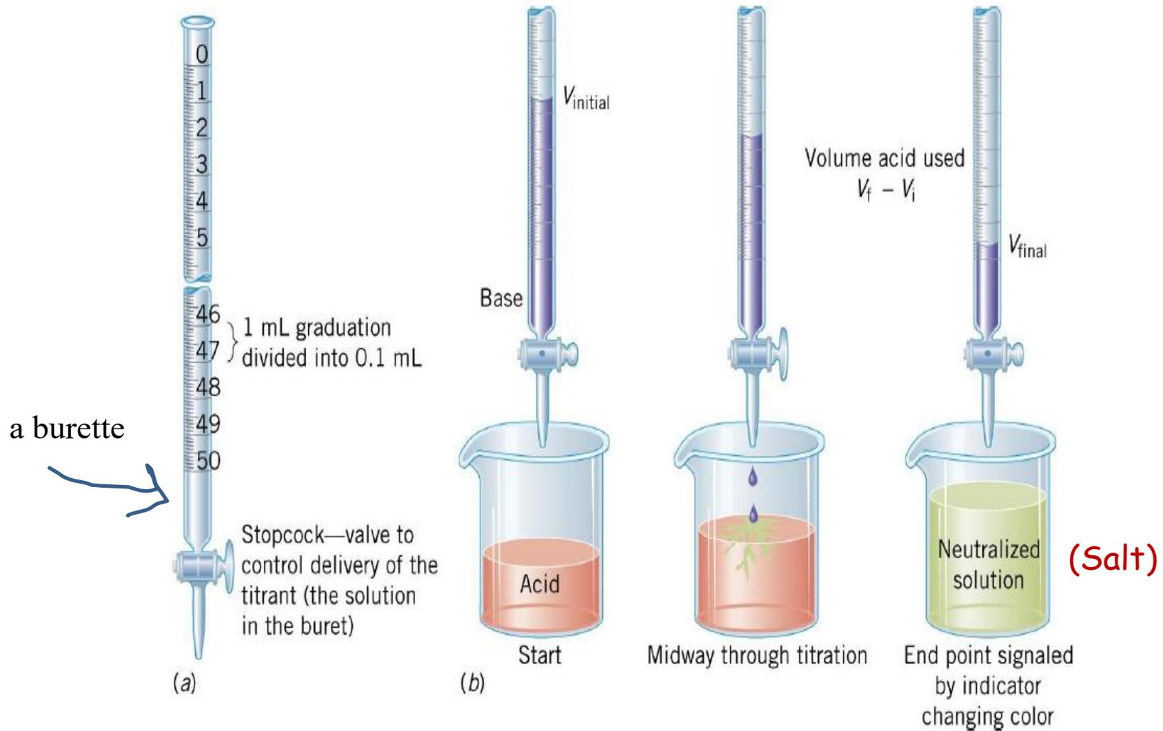
Titration of an acid solution of unknown concentration with a base solution of known concentration
